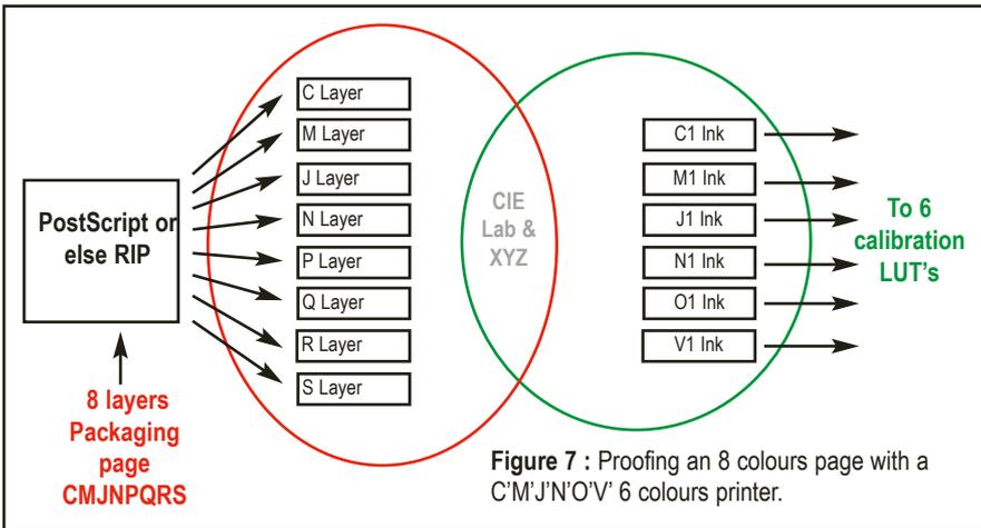
Figure 7 : Proofing an 8 colours page with a C'M'J'N'O'V' 6 colours printer.
