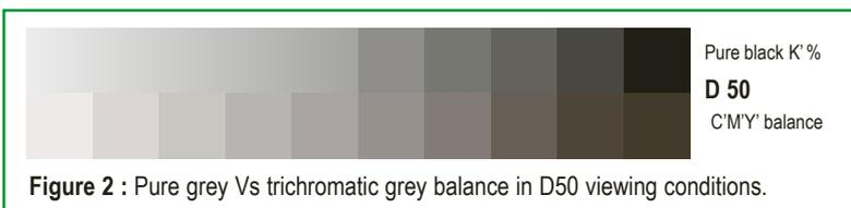
Figure 2 : Pure grey Vs trichromatic grey balance in D50 viewing conditions.
