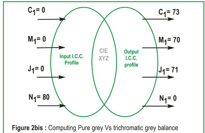
Figure 2bis : Computing Pure grey Vs trichromatic grey balance
