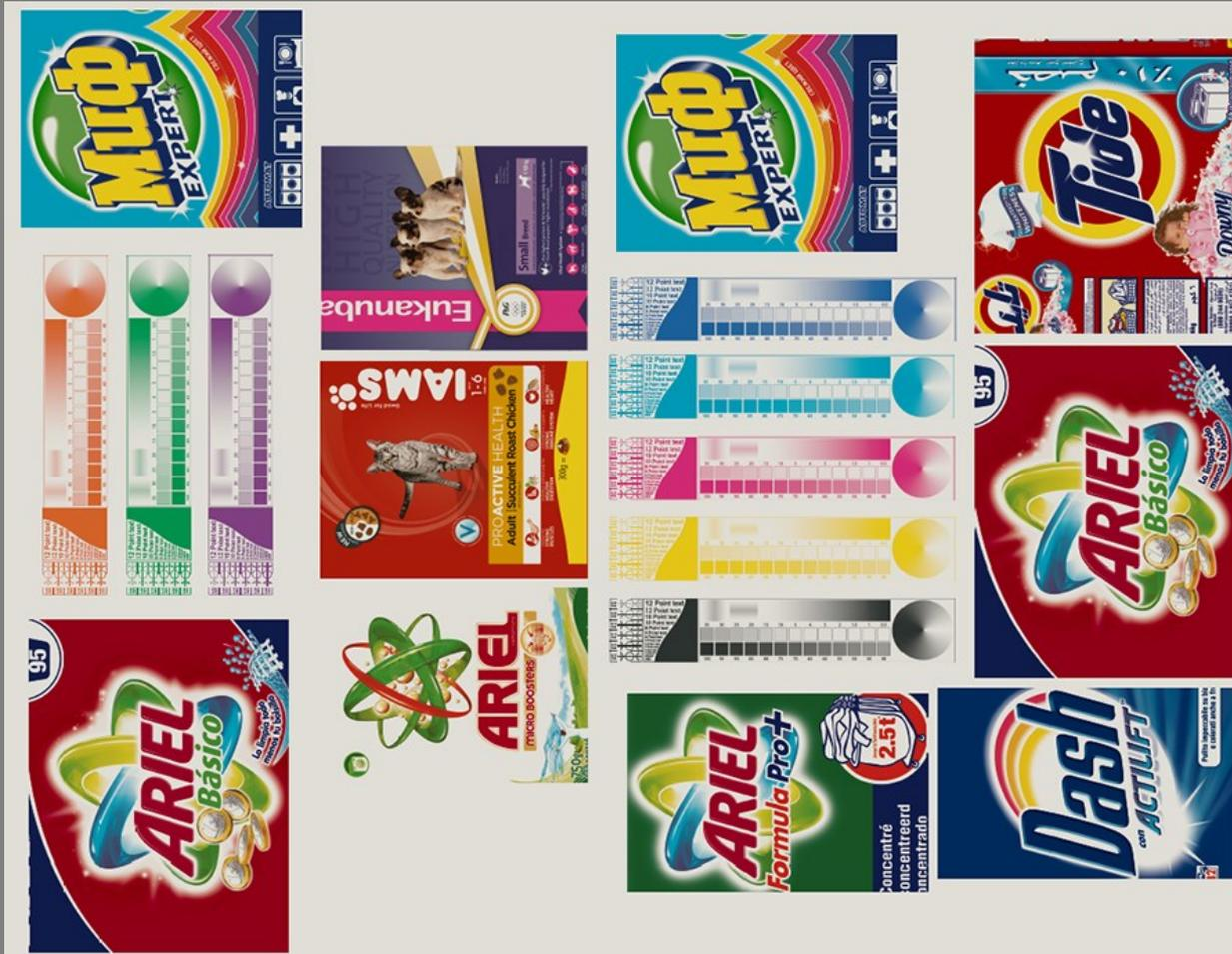
Solid inks colors AND their respective TVI curves, are the main parameters determining the final print job colors.
