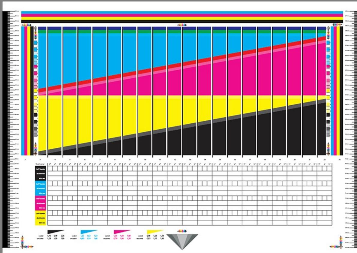
Example of a test form designed for manual search of optimal print densities, by impression with constant ink segments aperture on offset presses.
