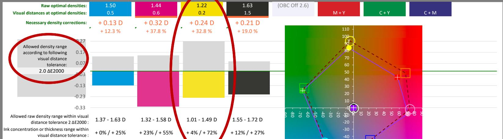
For a low 2 ΔE2000 tolerance, you can print **YELLOW** between 104% and 172% of the measured yellow ink thickness, i.e. make a **65%** ink thickness change!
