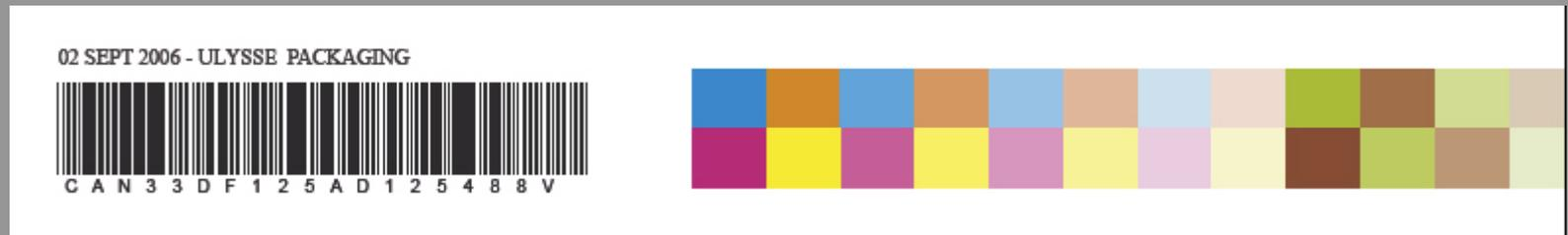
A software - downloadable on Internet - makes it possible to input the identifier met on any print or proof work, and get ALL useful information for fast, reliable and automated control of this control bar.
